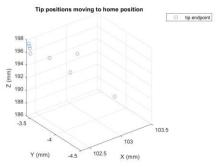
Using inverse kinematics and quintic task-space trajectory generation, we moved our robot between three locations in the X,Y,Z plane to visualize the accuracy of our model. As shown by graphs of the X,Y,Z position of the end-effector over time throughout the motion,
